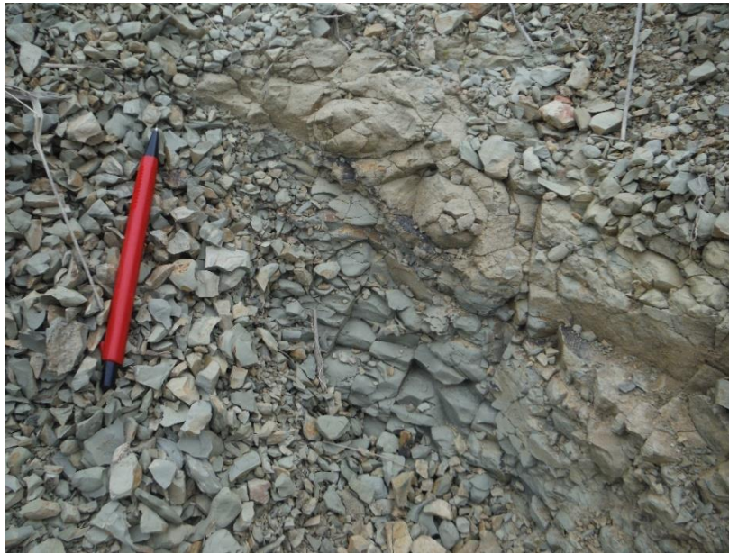
Figure A2.36 - Photo of the outcrop with layers of sandstone (Smm) and clayish siltstone (Fl).
