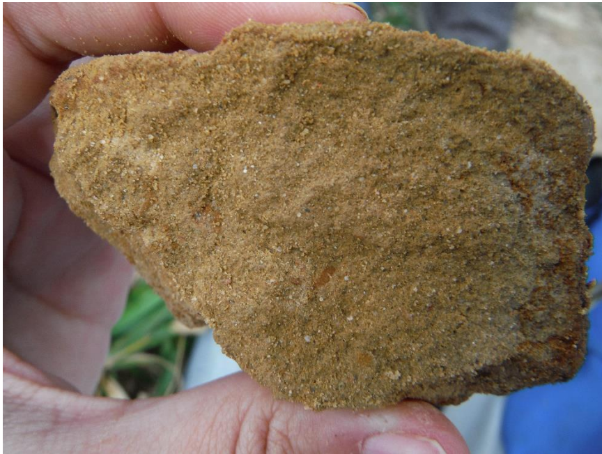
Figure A2.35 – Hand sample of fine, massive, immature sandstone, with matrix (Smm).
