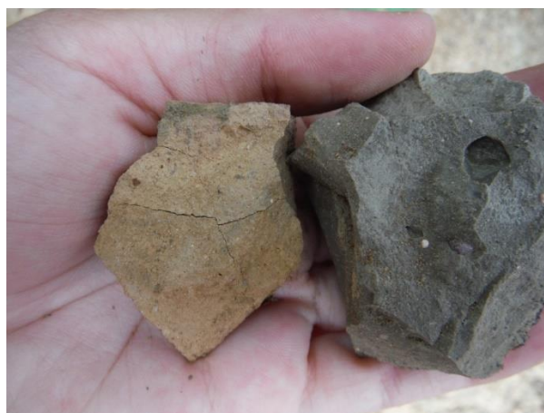
Figure A2.30 – Difference between the clayish diamictite (greyish yellow) (Df) and the sandy diamictite (grey) (Dm).
