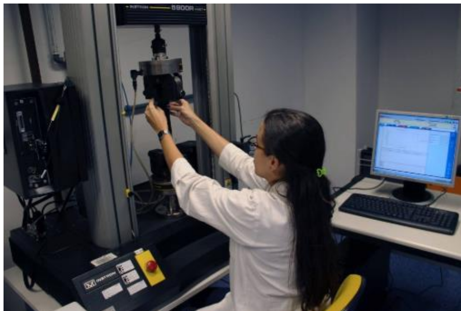
Source: Image https://senaicetiqt.com/tecnologia/metrologia/laboratorio-de-ensaios-fisicos/ Figure 4: Equipment for air permeability analysis. Rio de Janeiro, RJ, Brazil, 2020.
