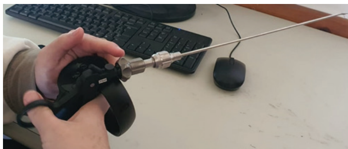
FIGURE 10. Revision to adapt clamp to Oculus control Quest II (source: by the author).
